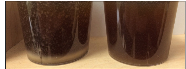
Picture of samples delivered for trial. Due to sedimentation of undissolved solids mechanical filtration (1 micron) has been performed before desalination test on electrodialysis.
